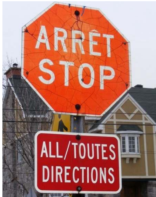
Image 7 and 8: 17-24-2464 and 22-10-393. On the left, we see significant rusting and weathering; on the right, cracking of the paint.
